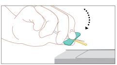
2. With the wing and shield between your thumb and index finger, press the safety shield against a hard surface such as a bedside table until an audible click is heard.
